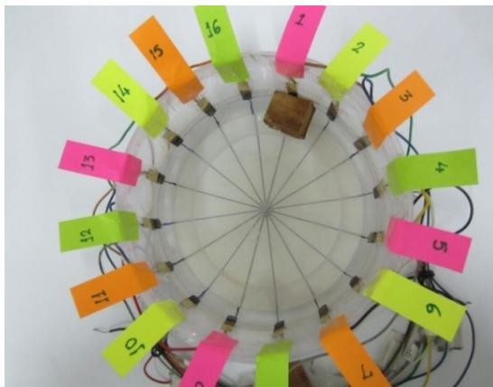
Fig 11: Container with non-conducting wooden impurity near
